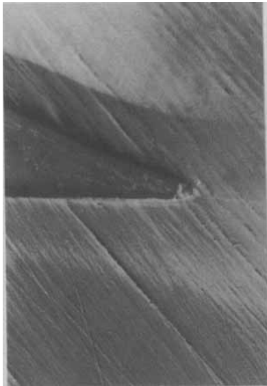
FIGURE 12 Typical crack path in the weld of a necked MEK solvent welded joint (magnification 100 \times ).
